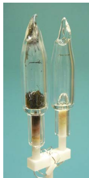
Figure 2. Homemade silica containers placed on a DTA sample holder. One silica container is charged with a mixture of WCl_6 and a reduction agent; the other (empty) one serves as a reference container.
